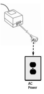
**Figure 4 –** 6 VDC power supply connection to AC power.
